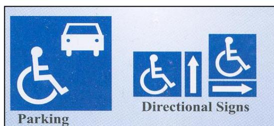
Figure 3-2. Signage for accessible parking
